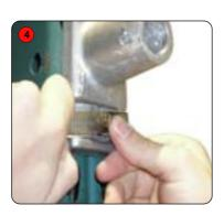
Push the screw down on the hose clamp to fasten it.
