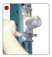
Pull on the hose clamp to tighten it.
