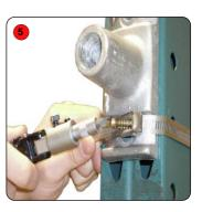
Tighten the hose clamp by turning the screw.
