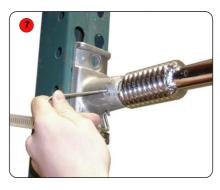
Push the safety pin through both holes to secure the pole in the pole mount
